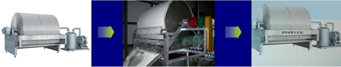
vacuum dewatering machine is domestic cassava starch production industry, yeast production industry Dehydration commonly used equipment, its manufacturing process is mature, mainly used for plant starch production in recent years Dehydration, degeneration starch production dehydration. In particular, the dehydration of potato and cassava starch emulsions is more reliable and more stable.
